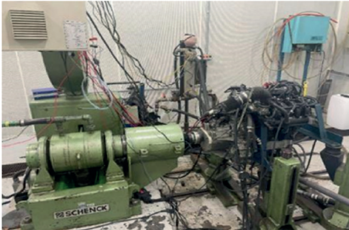
Figure 2 EA-111 VHT 1.6 l engine coupled to the dynamometer
