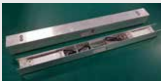
(8) Interior view of a weigh beam. A beehive is placed on two parallel weighing beams.
