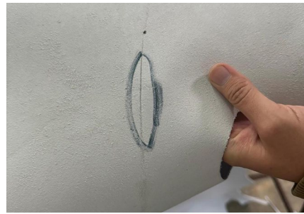
Fig. 3. Identification of leather defects prior to the cutting process.
