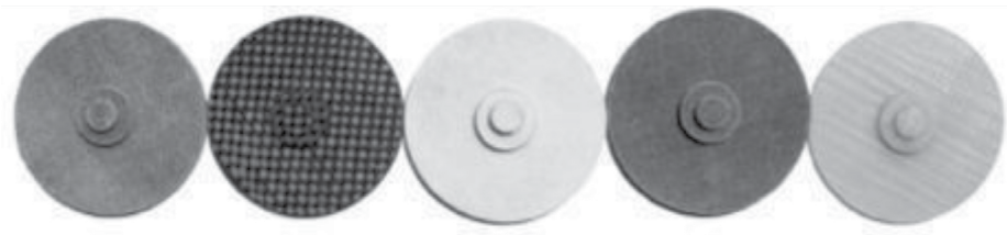
Fig. 7. Acoustic samples of composites with natural fibers [10].
