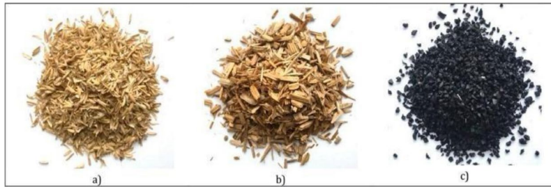
Fig. 5. Shows the materials used in the composites. (a) Rice husk. (b) Treated wood. (c) Recycled rubber [8].
